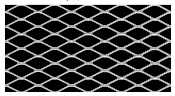
LW Pitch:30.48mmStrand Width:2.10mmSW Pitch:14.00mmThickness:1.50mmWeight:3.53 kg / m2Open Area:70%
